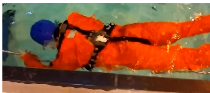
Figure 6: Hand-over-hand pull along bar: bar at 70cm; buoyancy of body means thorax and head are shallower – back of head is 'breaking surface', and depth of thorax/demand valve is shallower than 70cm.
