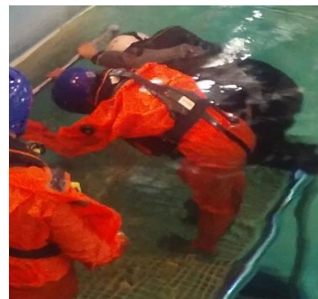
Figure 5: Breathe from EBS at ~50cms: head and thorax completely immersed
